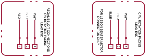
FIG. 1: WIRE COLORS - BASED ON INCOMING POWER
